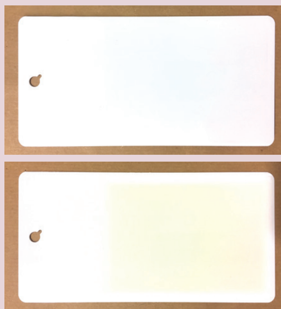
Comparison between the white versions of Awlgrip HDT (above) and an ordinary polyester topcoat (below). Awlgrip HDT shows almost zero signs of yellowing or discoloration.
